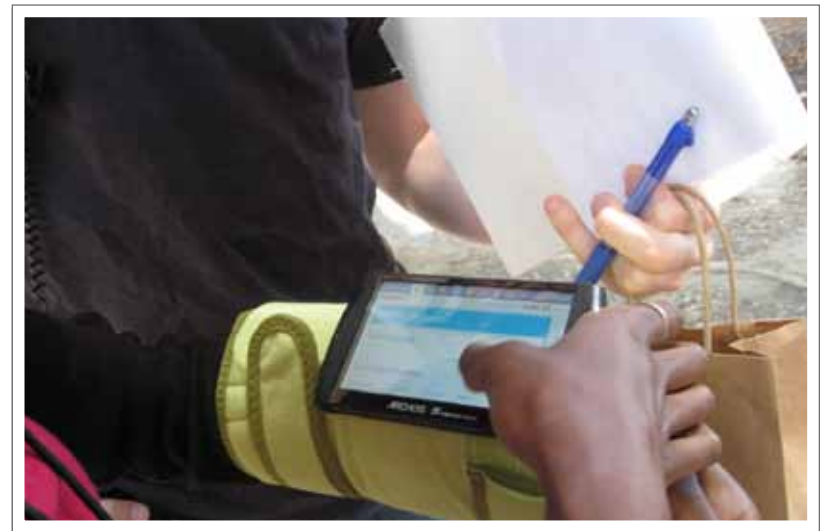
We used screen buttons for this ORT, which led participants to treat the entire device as a touch screen
