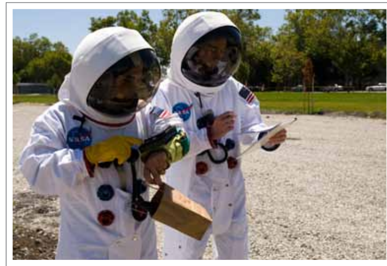
The cuff-mounted display frees the left hand for manipulating tools
