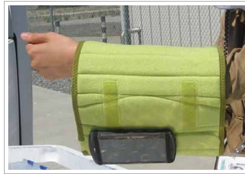
The Archos 5 device attached onto the arm brace using velcro and elastic
